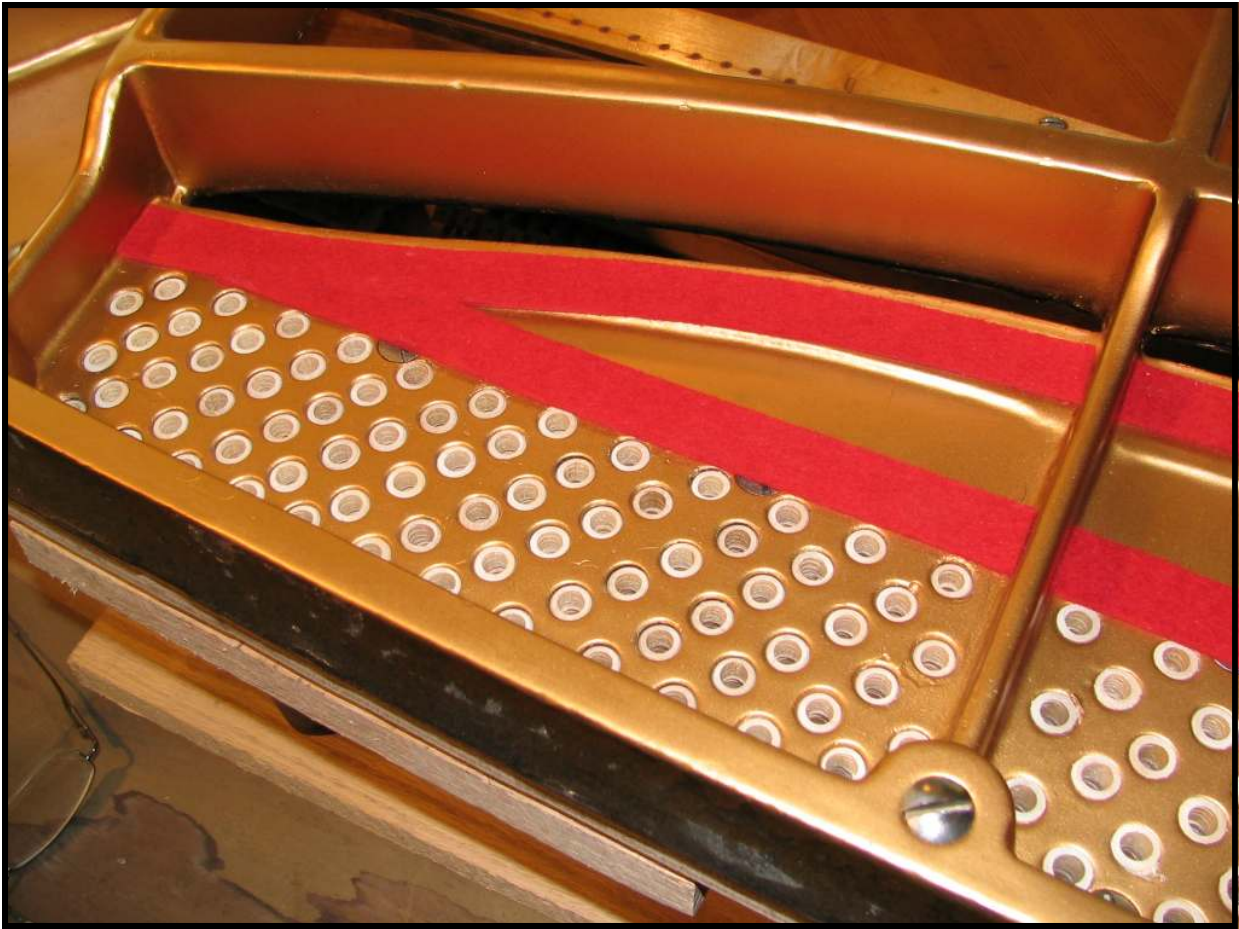
The new pinblock installed, ready for fresh tuning pins and strings.
